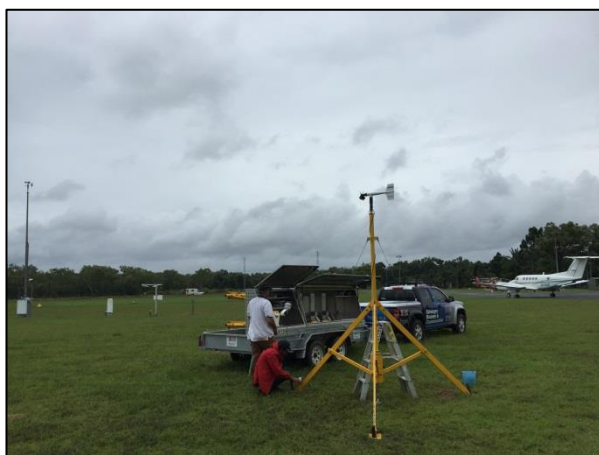
Figure 3. SWIRLnet anemometer Tower 1 (3 m height) and Cooktown Bureau of Meteorology (10 m height) automatic weather station (left hand side of figure) at the Cooktown Airport during TC Nathan.
