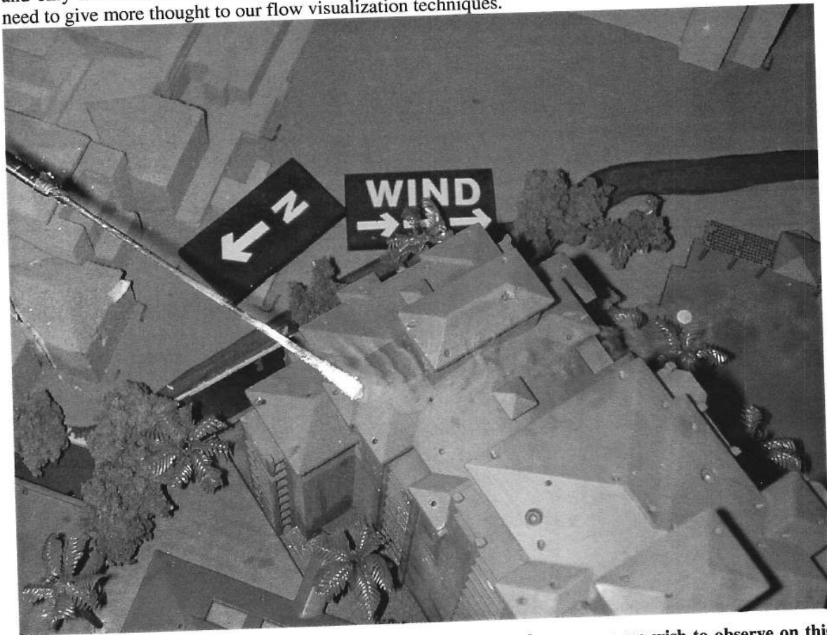
Figure 9: Flow shedding off the wand may influence the flow phenomenon we wish to observe on this Florida condominium. How much does the act of observing impact what we see?
