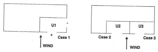
At specific locations within each unit that represent the location of operable portions of the façade, i.e. windows or doors, pressure sensors are placed, in addition to pressure sensors that are in place measuring the external pressure.
