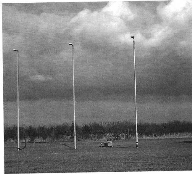
Figure 2. Experimental lighting columns at the Silsoe test site
