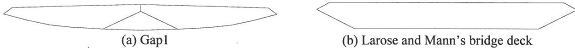
Fig. 2. The cross sections of Gap1 and that of Larose and Mann's bridge deck (of the same scale)
