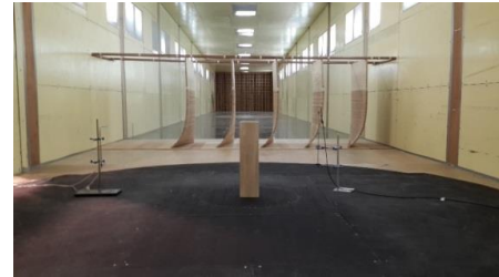
Figure 3. Building model and vane system set up in low wind speed section of boundary layer wind tunnel.
