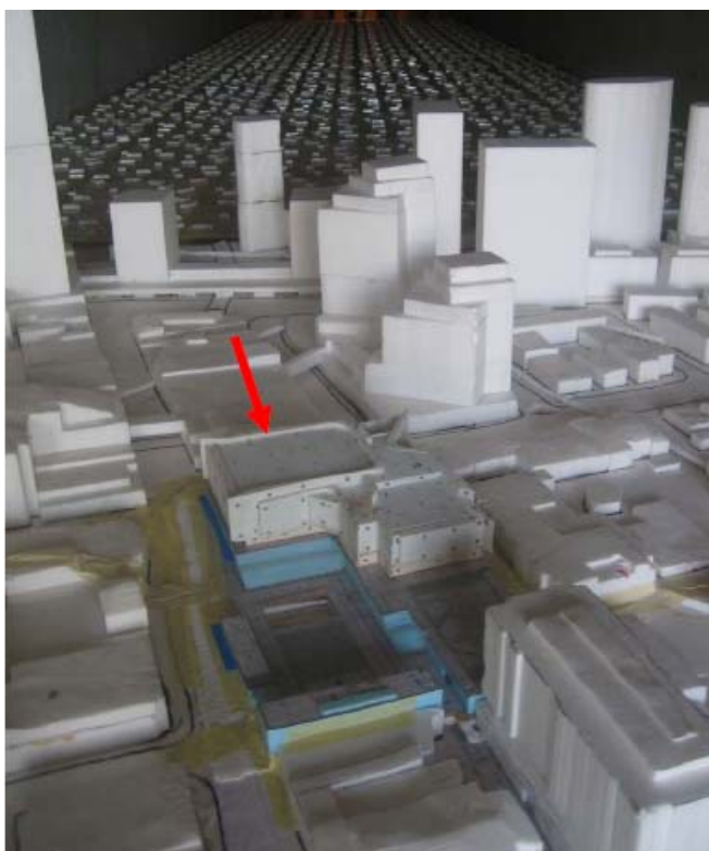
Fig. 1: Wind tunnel model for Chatswood Civic Place, Chatswood
