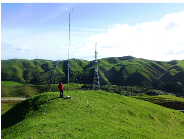
Figure 5. A NIWA 9 m tall anemometer mast installed at location Met6, looking towards the northwest and location Met9 which is at the highest point on the skyline.
