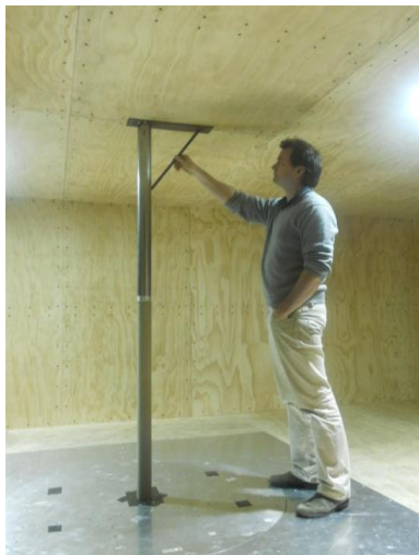
Figure 3. A circular cylinder set up for measurement of drag coefficient in the 1.5 MW Monash University wind tunnel
