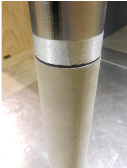
Figure 4. Close-up view of the gap between the upper (dummy) and lower (active) cylinders.
