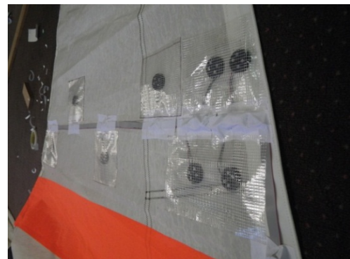
Figure 3. Differential pressure sensors on the sail
