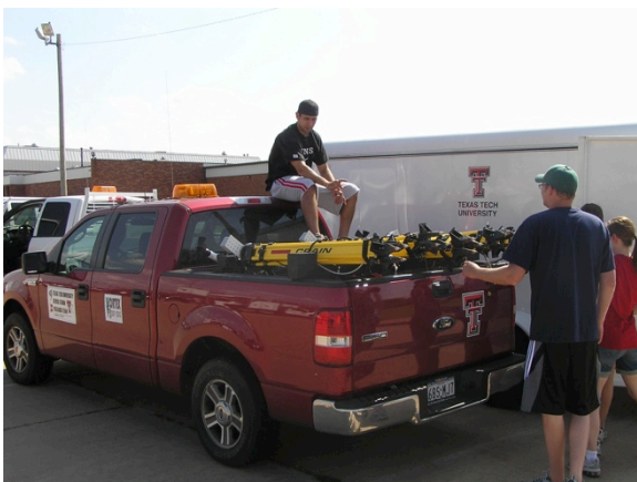
Figure 4. Five StickNet units mounted in the back of a pick-up truck for thunderstorm operations.
