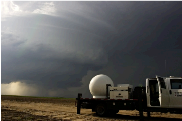
Figure 9. Photograph of TTUKa1 deployed nearby a supercell thunderstorm, showing the radome (rear), diesel generator (tan box) and auxiliary fuel tank (black box).
