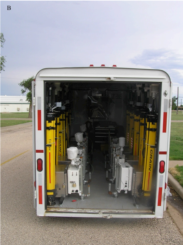
Figure 1. A third generation type “A” StickNet observational platform deployed in the thunderstorm configuration (A) and associated transport trailer (B).
