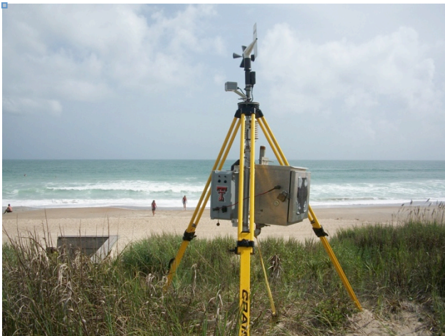
Figure 3. StickNet probe 0108A deployed on a sand dune for Hurricane Irene (2011).
