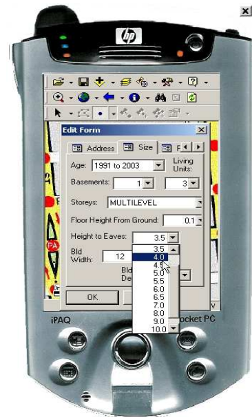
Figure 5. Image of PDA showing a single page of the survey template with the Height to Eaves field being entered from a drop-down list.
