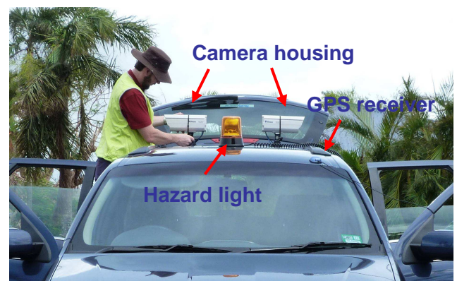
Figure 1. The RICS system mounted on a car. Images from the two cameras and positional data from the GPS receiver are automatically recorded on a laptop computer within the vehicle.
