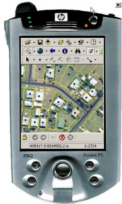
Figure 4. Image of PDA unit showing background image consisting of aerial photo, cadastral information, street layout and NEXIS points.
