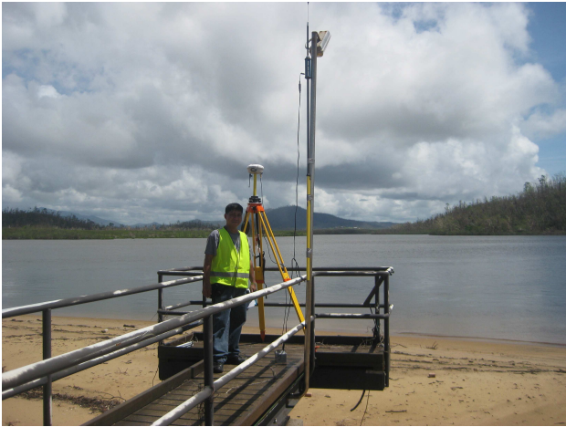
Figure 2. RTK survey equipment positioned over a permanent survey mark.
