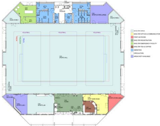
Figure 8. Proposed public cyclone shelter, Floor plan
