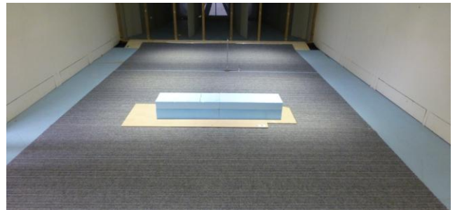
Figure 1. Photograph of 1/200 scale building model in the wind tunnel.
