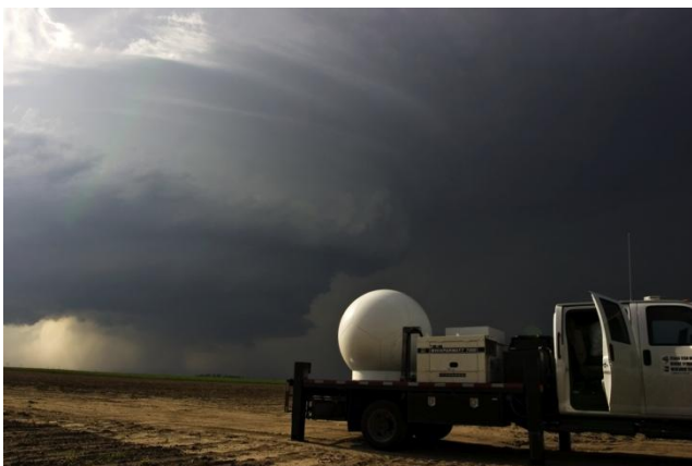
Figure 6. Texas Tech University Mobile Ka-Band Doppler Radars. Photo courtesy of John Schroeder
