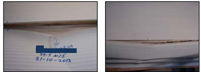
Figure 6. Impact location next to panel joint: front view (left); rear (right).
