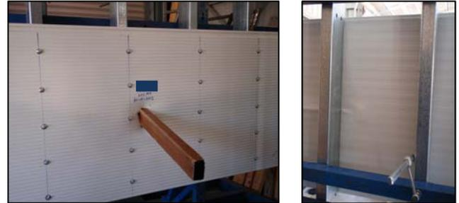
Figure 5. Impact location adjacent to support: front view (left); rear (right).
