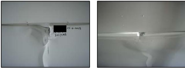
Figure 8. Impact location next to panel joint: front view (left); rear (right).
