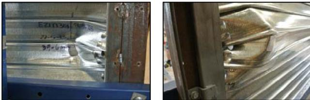
Figure 9. Impact location adjacent to support: front view (left); rear (right).
