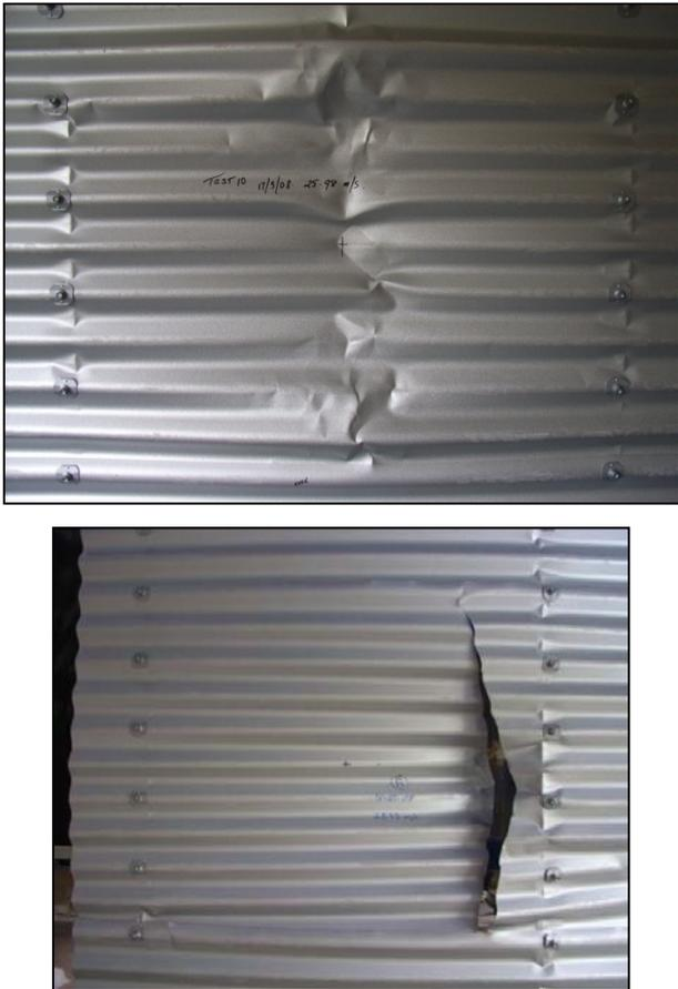
Figure 4. Corrugated wall cladding after impact at midspan (top) and close to internal support (bottom) by the 4 kg timber missile at 25 m/s. (Frye et al, 2012)
