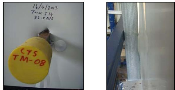
Figure 7. Impact location adjacent to support: front view (left); rear (right).
