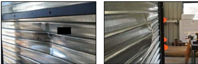
Figure 10. Impact location next to panel joint: front view (left); rear (right).
