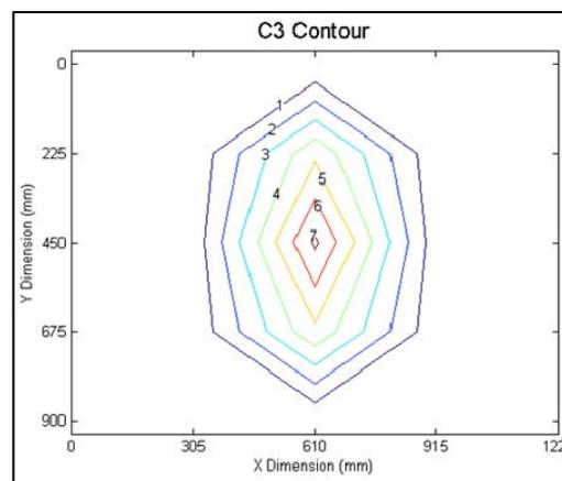
Figure 3. Cladding deflections (mm, absolute) in the z direction with loading at C1 (top), C2 (centre) and C3 (bottom). (Frye et al, 2012)
