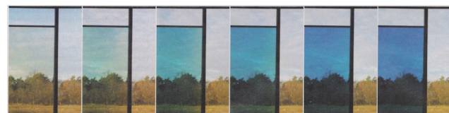
Figure 4. A window laminated with electrochromatic materials, tungsten oxide and Prussian blue, can be switched from transparent to dark blue as the voltage varies (after Mortimer, 2013).
