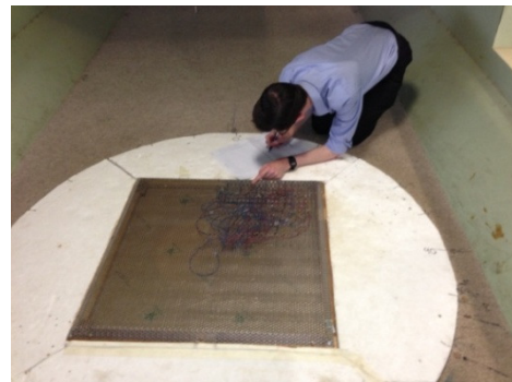
Figure 3. Model on turntable in wind tunnel
