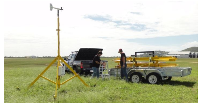
Figure 1. Tripod with anemometer deployed at Townsville airport. Note folded tripods in rack on trailer
