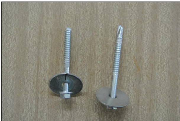
Figure 8. Photo image of tek screws after test
