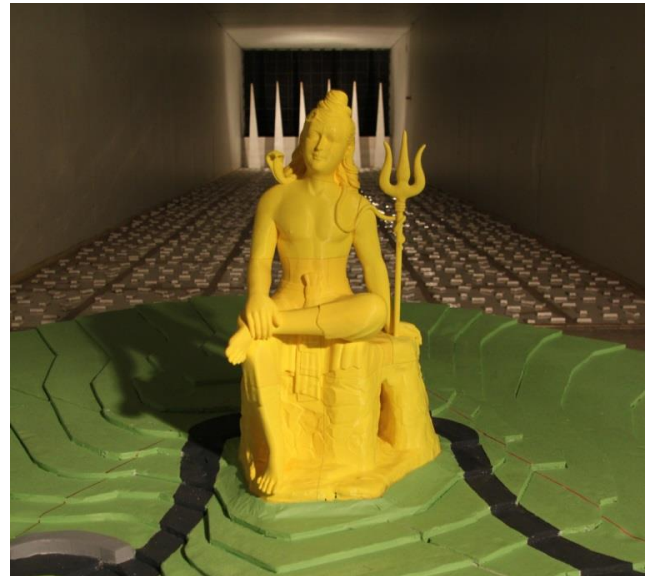
Figure 2: 1:200 Scale model setup in the wind tunnel
