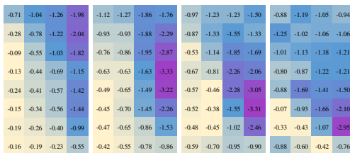
Figure 10 Successive time steps showing movement of peak load regions for wind direction 270°
