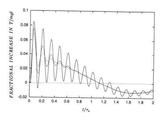
Figure 2. Plot of fractional increase in tension versus time for  $\delta t = 0.001$  (solid line),  $\delta t = 0.005$  (long dash line), and  $\delta t = 0.01$  (short dash line).
