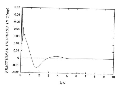
Figure 1. Plot of fractional increase in tension versus time for  $\delta t = 0.01$ .
