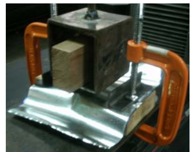
Figure 14 Combination of Roofing, Fastener, Purlin Test Set-up
