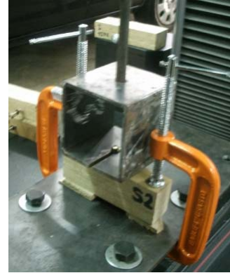
Figure 11. Single Fastener Test (Static Loading Set-up)
