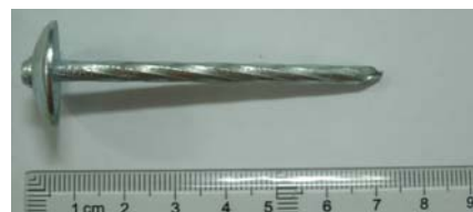
Figure 6. Wood Nail used in the experiment
