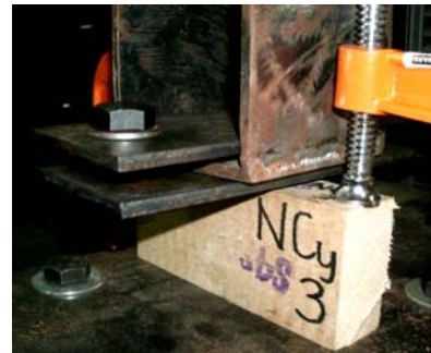
Figure 12. Single Fastener Test (Cyclic Loading Set-up)
