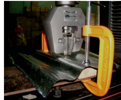
Figure 13. Static Loading for Roofing Test Set up
