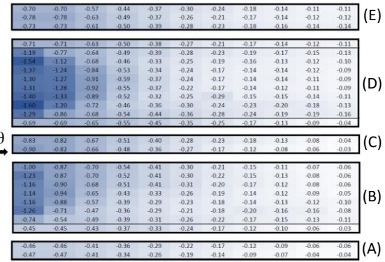
Figure 7: Mean C_p distribution for \theta = 90^\circ
