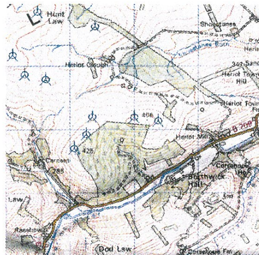
Figure 3: Sample windfarm layout map used in energy yield & noise optimisation software.
