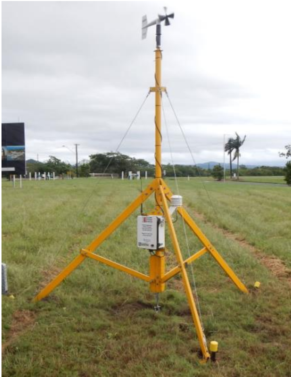
Figure 2. SWIRLnet tower with foot and central anchors shown.
