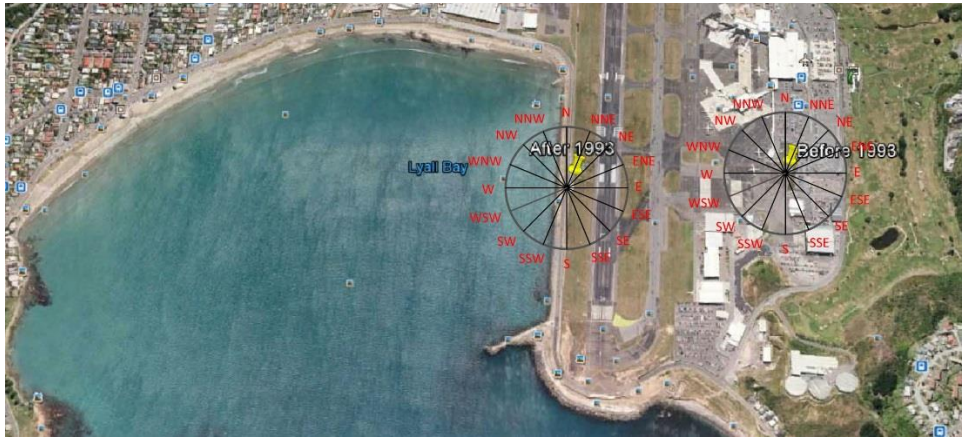
Fig. 1. The locations of anemometers at Wellington airport; (left) after 1993; (Right) before 1993
