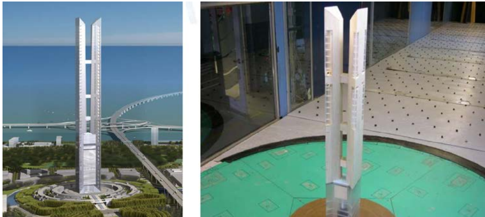
Figure 5 Incheon tower with side louvres shown on architectural and wind tunnel models – RWDI/Samsung
