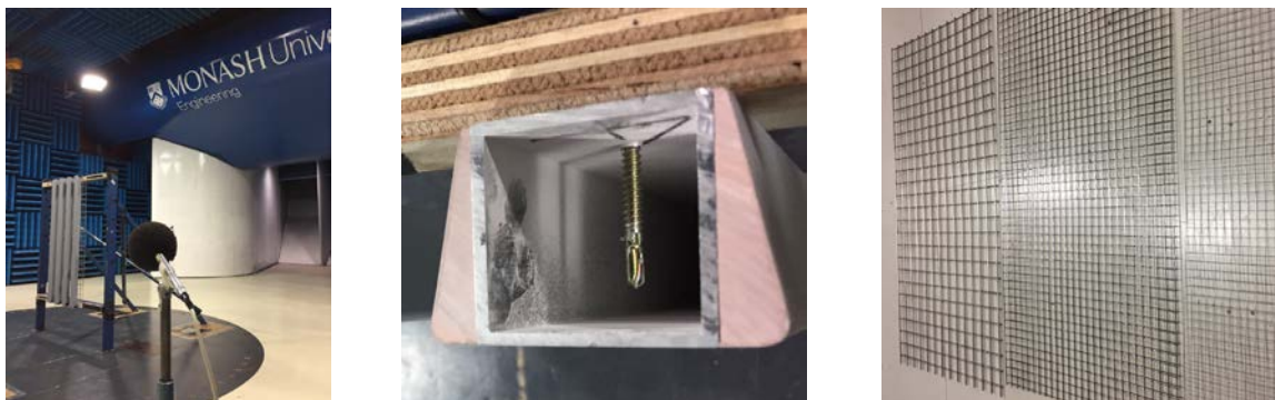
Figure 7 Wind tunnel setup, louvre section and mesh types tested
