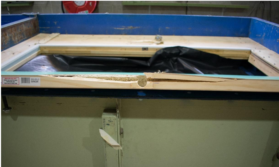
Figure 5. Split in timber of door in test 1, caused by door handle.
