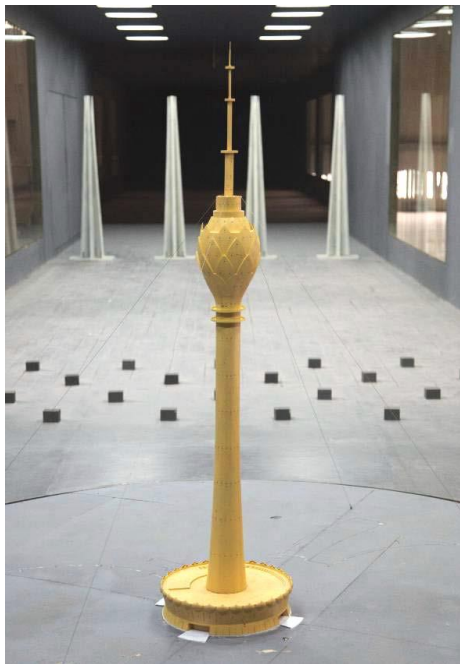
Figure 4: Wind Tunnel Tests prepared for the Lotus Tower
