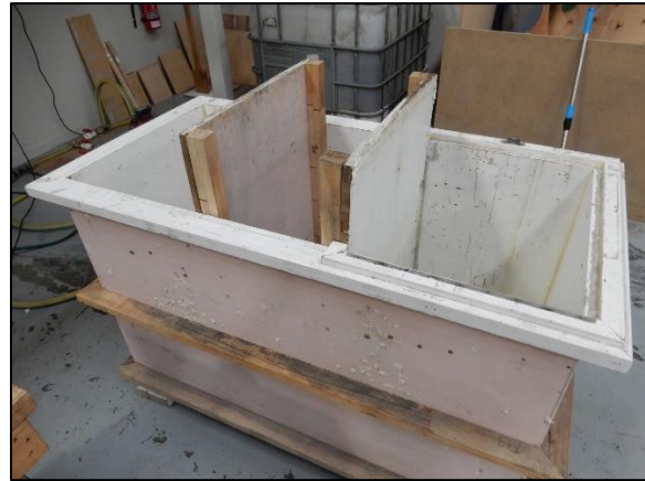
Fig. 6. Liquid tuned mass damper tank Fig. 7. Model of liquid tuned mass damper
