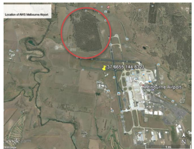
Figure 4. Melbourne Airport showing anemometer location (yellow 'pin') and forest of trees to the north west (red circle)
