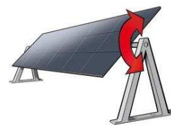
Figure 5: Typical solar tracking ground mounted array
