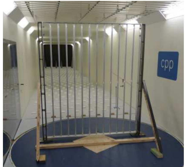
Figure 4: 2 m high full-scale fence in the wind-tunnel
