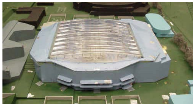
Fig 9, 10 Wimbledon Centre Court Closing Roof – Wind tunnel test model, roof closed, roof open load case below. BMT Fluid Mechanics
