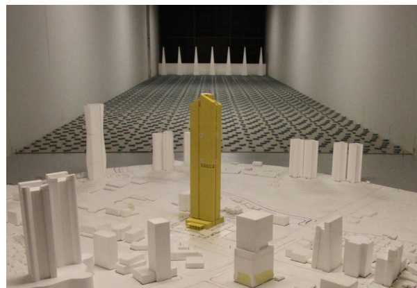
Figure 1. The wind tunnel test model (October 2010) in Windtech's Boundary Layer Wind Tunnel Facility.
