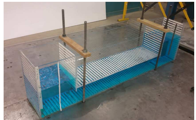
Figure 5. Shake table test of the 1:10 scale TLCD model (without TLSD, without mesh panels).
