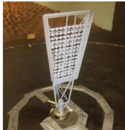
Figure 15 HFBB measurements of drag coefficient
