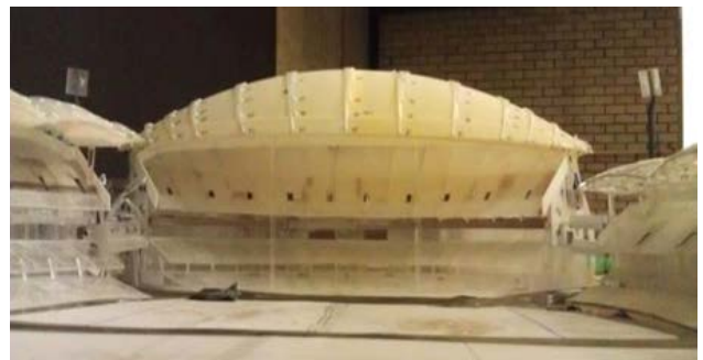
Figure 9 Wind tunnel model at 1:200 scale generated from 3D print
