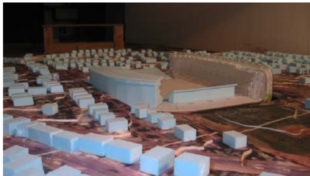
Figure 5 Eden Park Wind Tunnel Test
