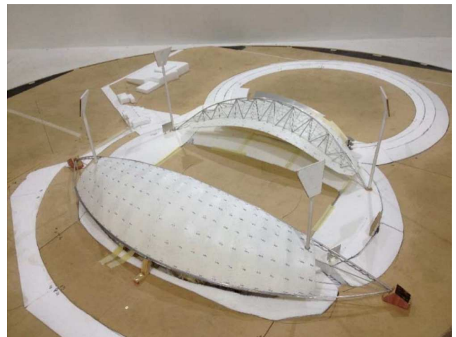
Figure 1. View of wind tunnel model with new canopy in foreground with the exterior pressure taps visible.
