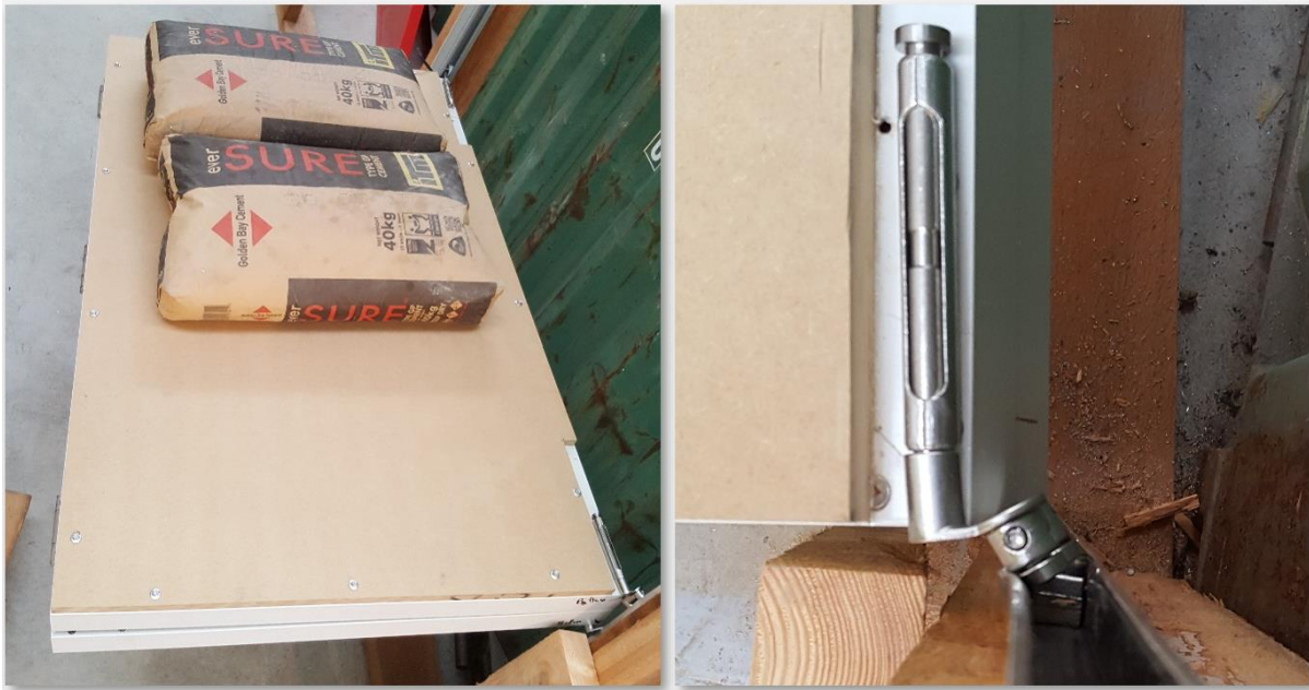
Figure 2. Bi-fold hardware load testing.
