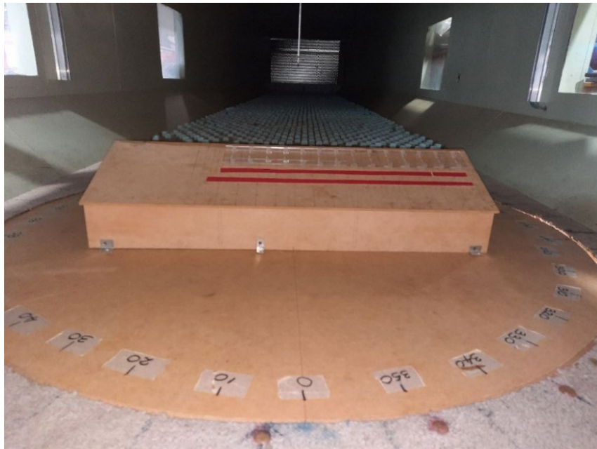
Figure 1. Wind tunnel model in the boundary layer wind tunnel
