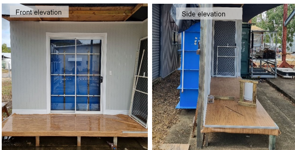
Figure 1. Wind driven rain simulator test apparatus
