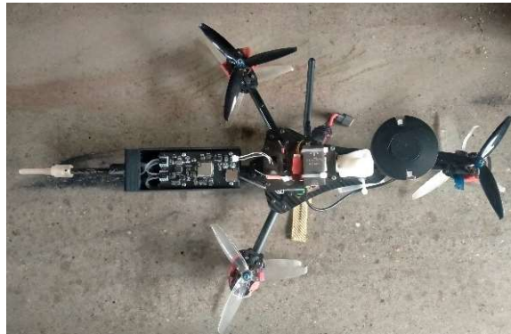
Figure 5. A hexa-rotor drone with multi-hole anemometer system
