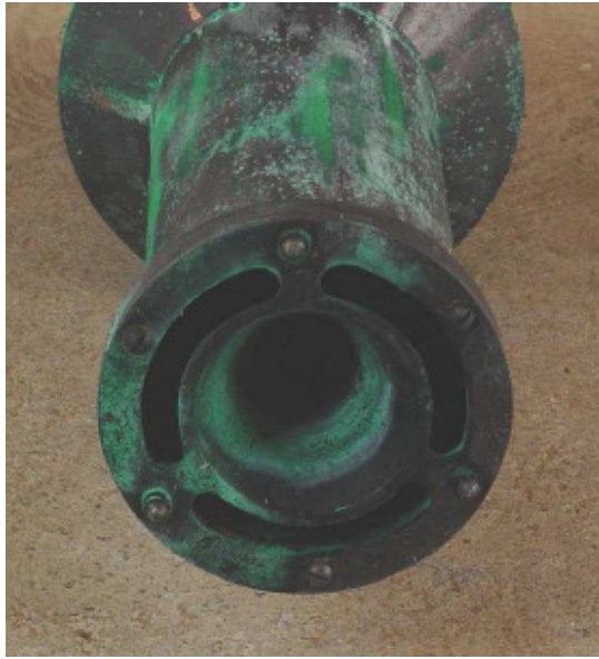
Figure 5: Photograph of the lower end of a Dines anemometer float, showing the choke. The pressure tube enters up the hole in the middle, almost filling it.
