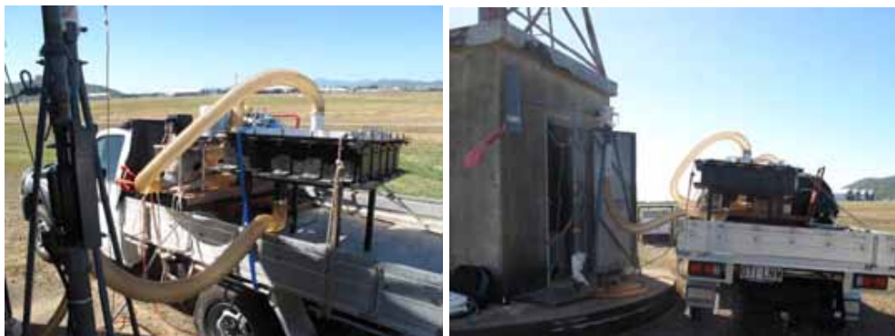
Fig. 1: (a) PLA connected to volume chamber which is connected to Dines; (b) PLA system connected to Dines head in doorway (with 3 phase generator in background)
