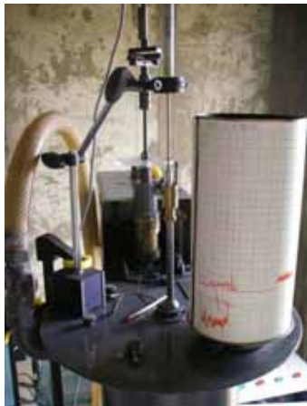
Fig. 2: (a) LVDT connected to modified shot-cup on top of float rod; (b) Plot of vertical movement of float rod (measured by LVDT) with derived "wind speed" converted from applied PLA pressure
