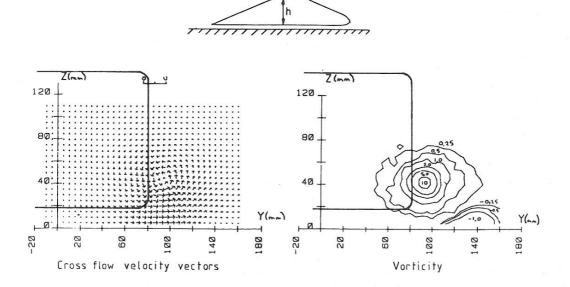
Figure 1. Wake survey behind 25 deg slanting base at x/h = 6.5, ground clearance = 0.15h.
